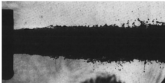
FIG. 14: Near-nozzle photograph of a water jet in the turbulent surface breakup regime from Wu et al. (1995, fig. 5c). Flow is from left to right.
