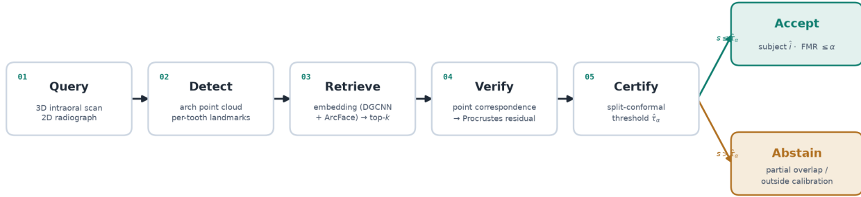
Figure 1: The unified ToothPrint pipeline. A query is detected into an arch point cloud or per-tooth landmarks, retrieved against the gallery by a global embedding, verified on the shortlist by learned point correspondence with a rigid Procrustes residual, and certified by a split-conformal threshold \hat{\tau}_\alpha : the nearest candidate is accepted as subject \hat{i} only if its score clears the threshold (false-match rate \leq \alpha ), otherwise the system abstains.
