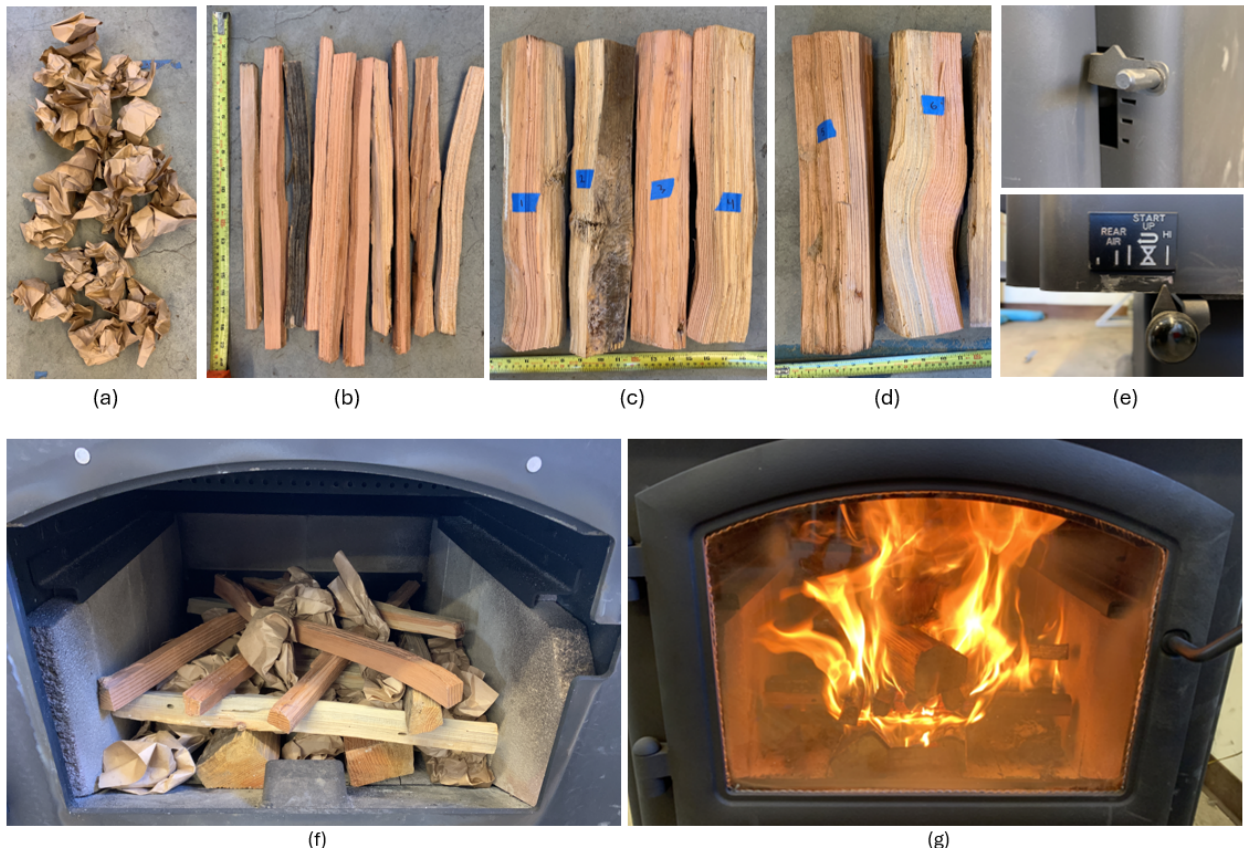
Figure S2: Images of the cordwood heater high-burn phase paper knots (a), kindling (b), small fuel logs (c), large fuel logs (d), air-control settings (e), firebox before lighting (f), and firebox after all fuel is loaded (g).
