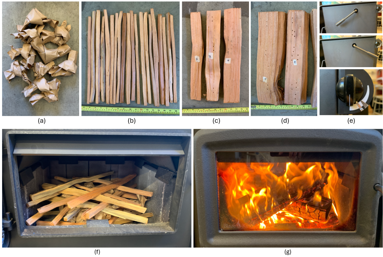
Figure S4: Images of the catalytic-cordwood heater high-burn phase paper knots (a), kindling (b), small fuel logs (c), large fuel logs (d), air-control settings (e), firebox before lighting (f), and firebox after all fuel is loaded (g).
