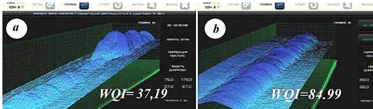
Figure 3. Indices for evaluating the practical skills of welders.: WQI = 37.19 (a), WQI = 84.99 (b).
