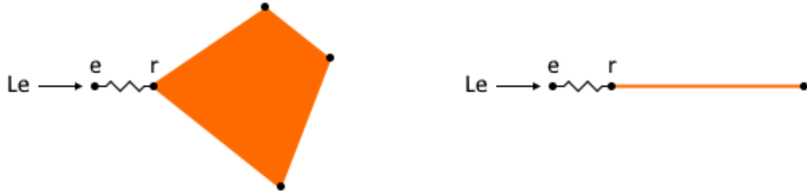
Figure 2 – External Node Added and Internal Spring Changed to External
