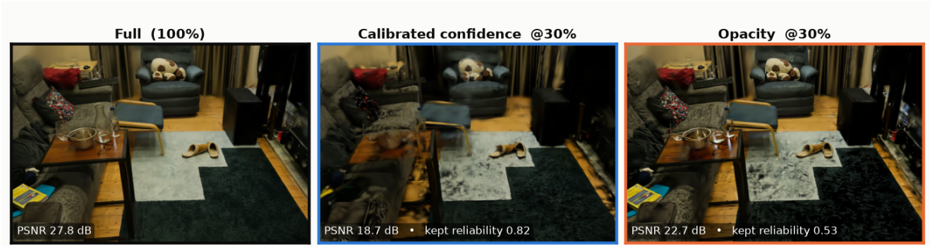
Figure 8: RQ3 (qualitative): pruning to 30% of carriers on a held-out Room view. Left, the full asset; centre, keeping the top 30% by calibrated confidence ; right, keeping the top 30% by opacity (the engine default). Each panel is annotated with its render PSNR against the ground-truth image and, for the pruned panels, the mean held-out reliability of the kept set. This single view illustrates the aggregate trade-off of Fig. 7 and Table 9: opacity — being the alpha-composite blend weight — preserves the render (22.7 dB vs. confidence’s 18.7 dB) but keeps unreliable carriers (retained reliability 0.53), while calibrated confidence keeps the reliable ones (0.82) at the cost of PSNR. This is the 30%-keep operating point of those curves; it is not a PSNR claim (Sec. 9.3: opacity is the render-preserving prune). Committed artifact repo/assets/pruning_30pct.png, generated by experiments/make_pruning_sweep_gif.py (calibrator fit exactly as calibrate_confidence.py , seed 0).
