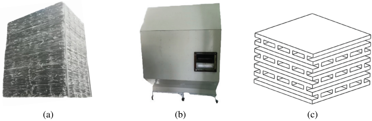
Figure 4: (a) Manufactured heat and mass exchanger, (b) Packaged Dew-point cooler using the heat and mass exchanger, (c) illustration of laid up sheets allowing cross flow of wet and dry channels.
