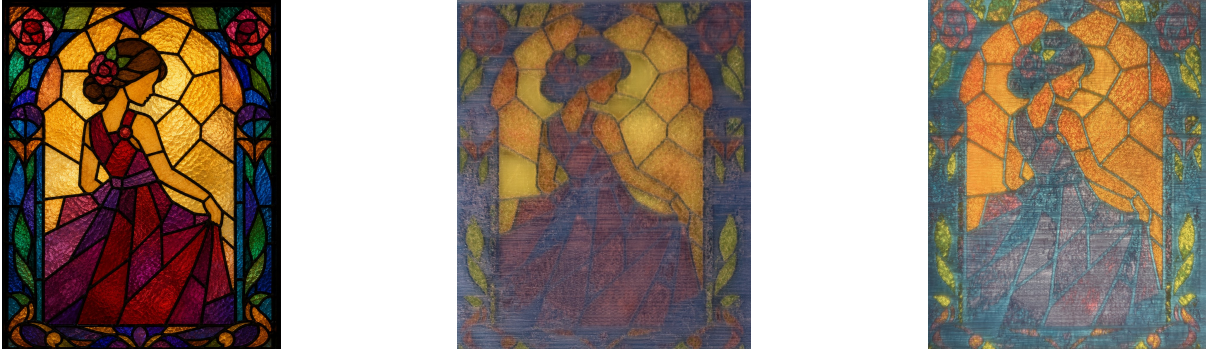
Figure 6: Application print. Source image (left), the printed translucent layered CMYW panel front-lit (center), and the same panel backlit (right), where subtractive transmission through the stacked filaments yields saturated stained-glass color.
