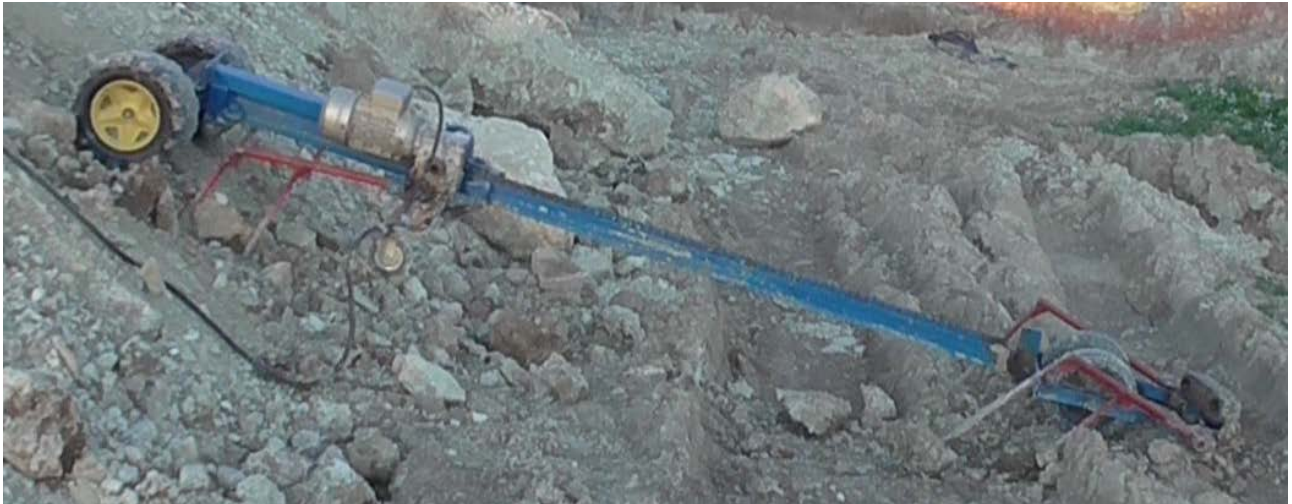
Fig 13: At the bottom of the far side another concavity is overcome. Note how the vehicle has sufficient traction to push through obstructing ridges of soil at the bottom of the mound.
