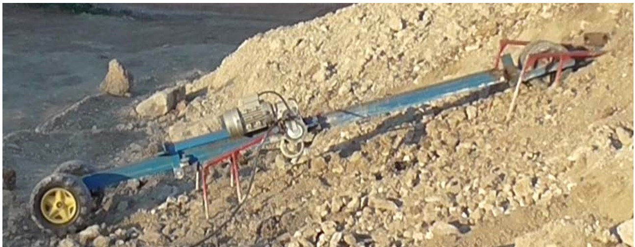
Fig. 9: UTOPUS has overcome the concavity. As it climbs it pushes obstructing gravel and rocks aside. Note that rock fragments tend to accumulate on the surface of debris flows due to granular convection.
