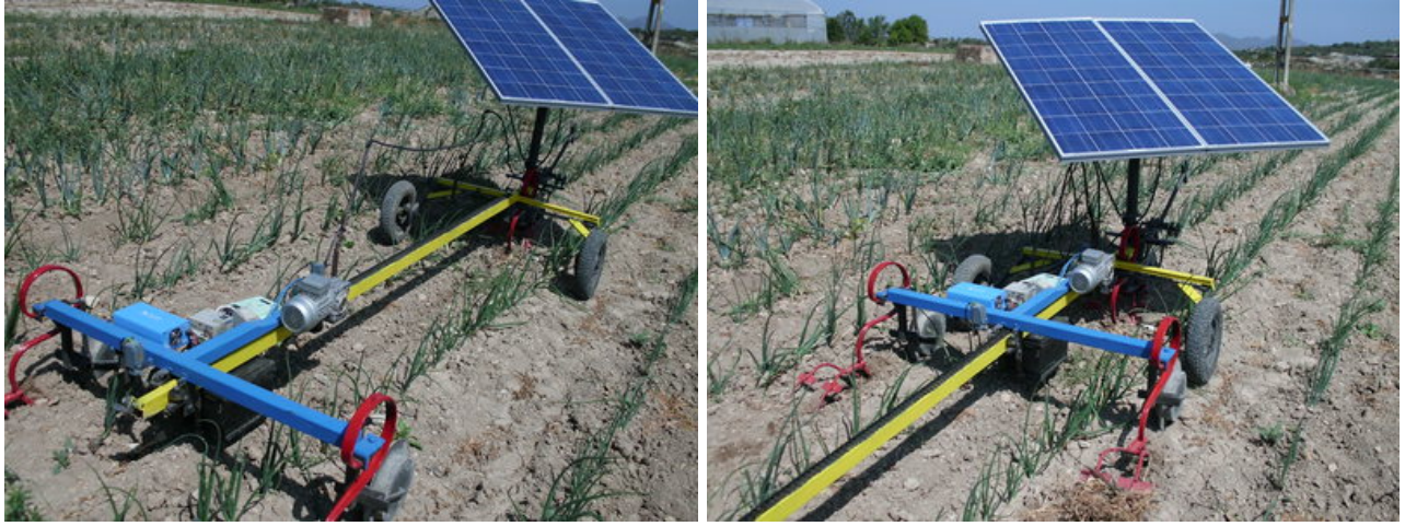
Fig. 3. An agricultural version of UTOPUS cultivating an onion field with energy autarky. In the images the vehicle moves from bottom left to upper right. Left: During the pull phase the back frame (left) advances while the crampons of the front frame (right) have been driven into the ground and provide traction. Right: At the start of the push phase the crampons of the back frame are driven into the ground, allowing the front frame to advance.
