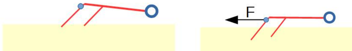
Fig. 5. Crampon design. The hinge at the back of the frame is indicated by a blue circle. Left: The crampon before entering the ground. Right: The crampon anchored in the ground, resisting the drawbar pull F .
