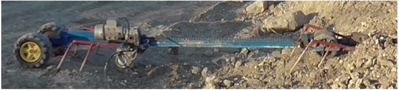
Fig. 7. At the beginning of a climb UTOPUS pushes the shaft into the mound. The crampons generate sufficient traction to allow the vehicle to align itself with the new axis of advance.
