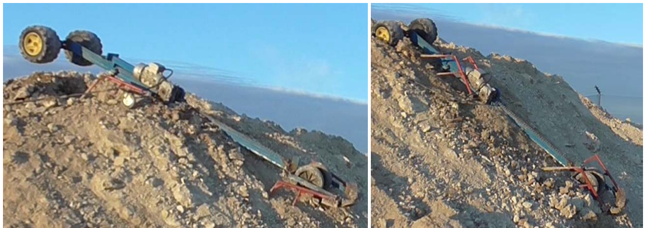
Fig. 12. UTOPUS has overcome the top ridge and starts to descend on the far side. Left: As UTOPUS descends, its rear end is momentarily lifted into the air and the shaft slides over and through the ground without any noticeable consequences. Right: Where moving parts touch the ground, small avalanches are created. The crampons keep the vehicle stable and it never slips.
