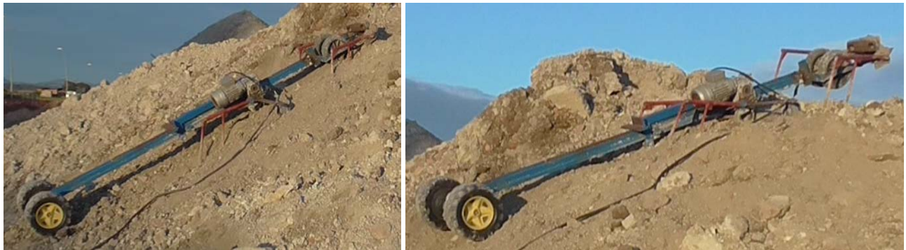
Fig. 10. Left: UTOPUS in full climb. Right: Reaching the top, the front end is temporarily suspended in the air. A 4 kg iron ballast is visible on top of the front end.
