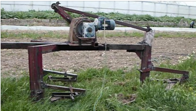
Figure 11: Left: UTOPUS for deeper tillage (20 cm), March 2012. Right: Wind powered design, June 2012.
