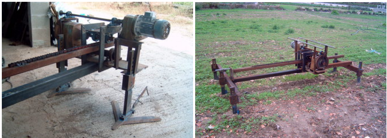
Fig. 8: Left: Improved crampon design, July 2010. Right: Improved stability, September 2010.
