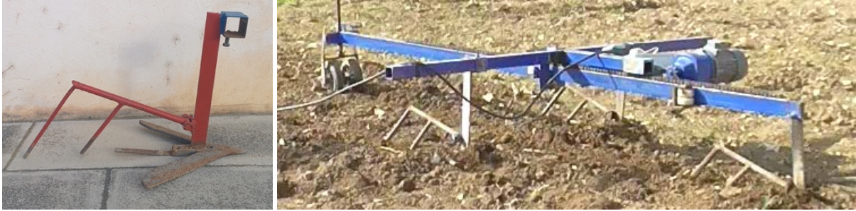
Figure 1. Left: Set of spikes with lever arm and movable joint, attached to the rear of a tillage tool. Right: Tillage device with one set of spikes and tillage tool in front of the main frame, and two sets of spikes and tillage tools on either side of the sliding frame. In the photo, the device moves from left to right and the horizontal draft force on the spikes from the tillage tools is directed from right to left.
