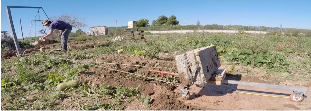
Figure 4: The actual experiment, here in a pumpkin field after harvest, in wet soil. We attached the basket with bricks to the left to a cable, which pulls the device to the right. Note the concrete block on top of the device, without which the device would rotate about the tip of the spike in the soil.
