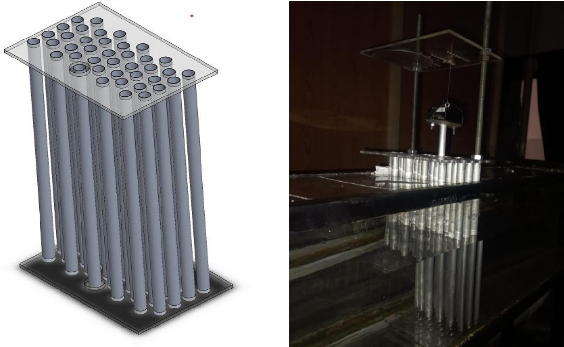
FIGURE 8-1 TUBE BUNDLE MODEL VIEW(LEFT) AND EXPERIMENTAL SETUP(RIGHT)
