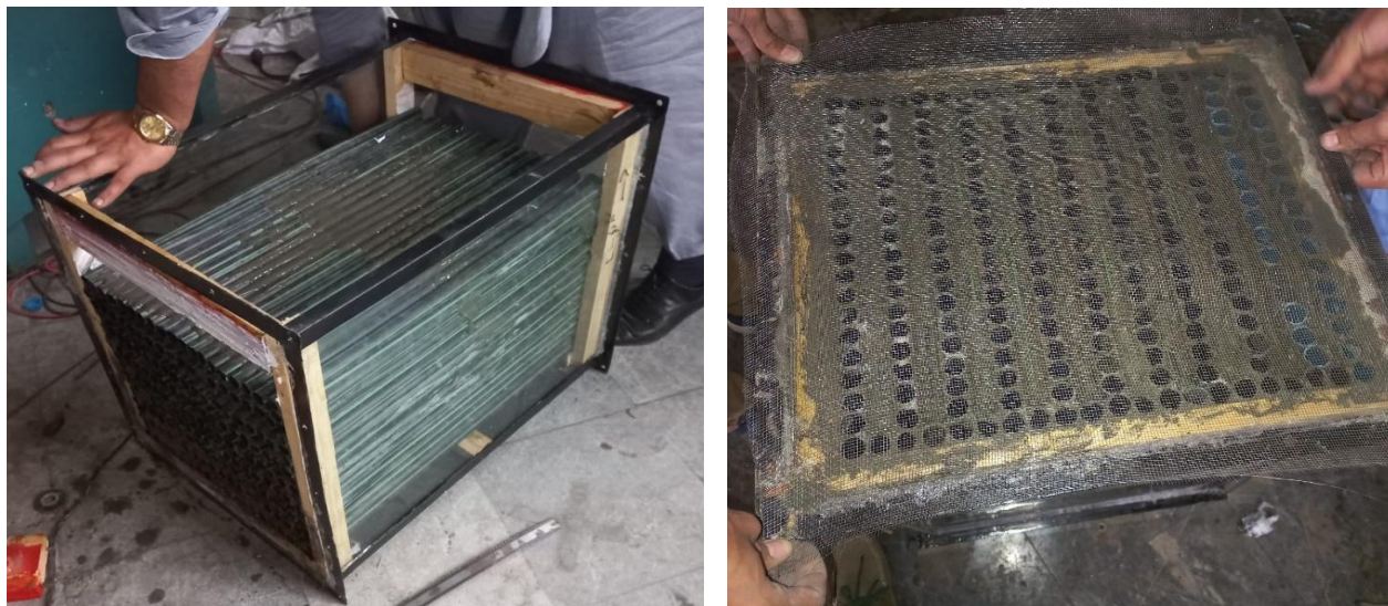
FIGURE 7-1 FABRICATION PROCEDURE OF BAFFLES
