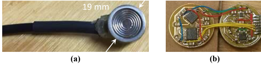
Figure 3. Earth pressure cell: (a) Plan view; (b) Internal 3-axis accelerometers.
