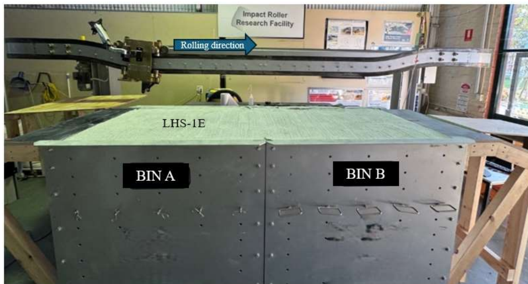
Figure 1. Scale model test rig showing the test bins filled LHS-1E and the chain-driven carriage system used to mobilise the LVDR-2 model.
