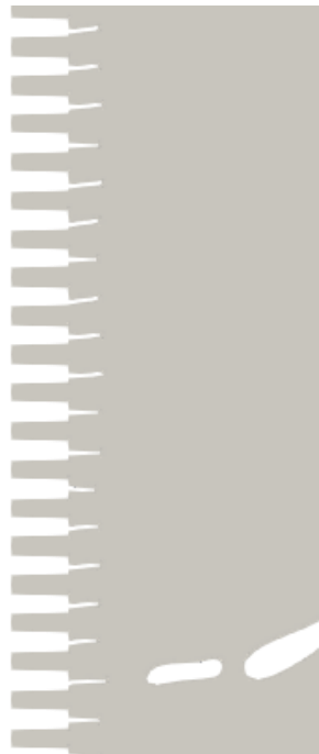
Figure 5.10: ColdStream's inlet structures
