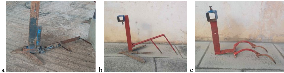
Figure 2. Empirical crampon designs. In each photo, there is a vertical shaft that connects the crampon to its implement frame. At the base of the shaft, there is a horizontal hinge to which the crampons are connected, allowing them to swing up and down. The straight crampons in (a) and (b) penetrate the soil to a depth of 10cm and 20cm respectively, the curved crampons in (c) penetrates to about 5cm. (a) and (b) also have a tillage implement (a sweep) connected to the base.
