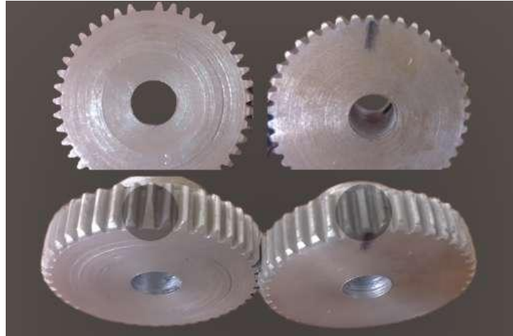
Figure 2: Two defective gears with Edge Broken, left side, and Half Tooth Broken, on the right side
