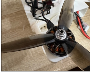
Figure 30: Motor with Propeller Secured onto Drone Arm with Wires through Guidance Hole
