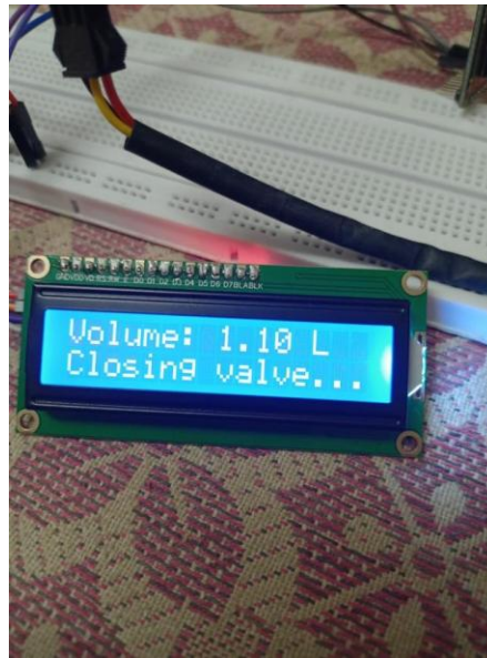
Figure 4. Prototype LCD showing a valve-closing state at a configured test condition (project photograph).
