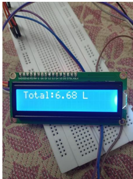
Figure 2. Prototype LCD showing accumulated water volume of 6.68 L during testing (project photograph).
