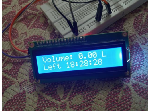
Figure 3. Prototype LCD at a 0.00 L display state with time information (project photograph).
