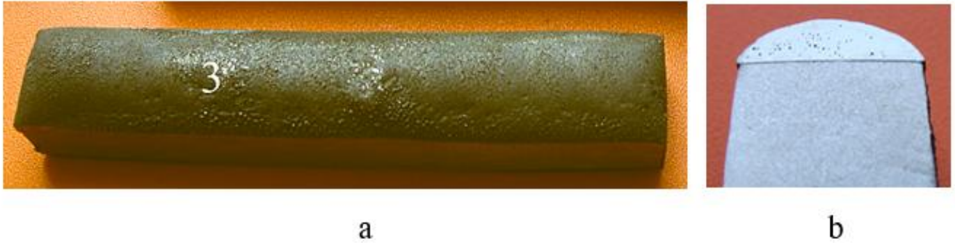
Figure 12. Sample of a weld bead probe from PG-10N-01 powder (a) and its macrosection (b).
