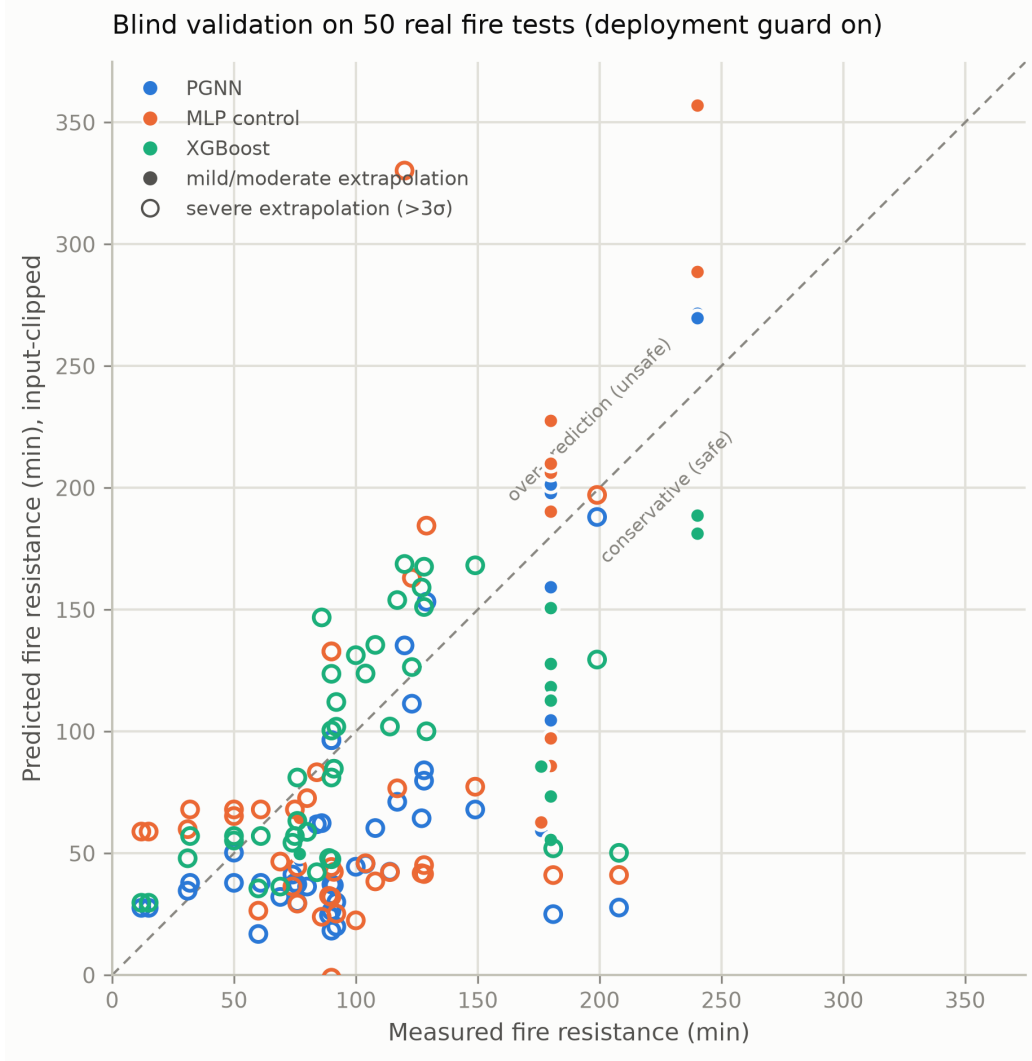
Figure 8: Parity plot of predicted vs. measured fire resistance (FR) under the input-clipping deployment guard, for three representative models (PGNN, MLP control, XGBoost). Markers are coded by extrapolation severity: filled markers denote beams within the mild or moderate strata ( s \leq 3\sigma , n = 10 combined), and open circles denote the severe stratum ( s > 3\sigma , n = 40 ); see Table 8 for metrics computed separately on the moderate and severe strata. The dashed diagonal is the line of perfect prediction; points above it are unsafe over-predictions, points below it are conservative.
