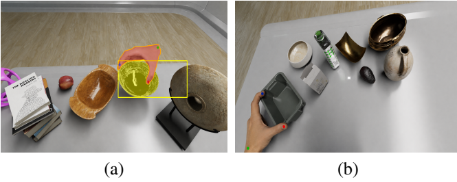
Fig. 6: Failure case examples. (a) Bowl: SAM3 bounding box exceeds object limits causing misplacement of mapped points. (b) Oil Tin: GPT-5.6 Luna incorrectly generated a grasping configuration for a plastic container instead of the oil tin.
