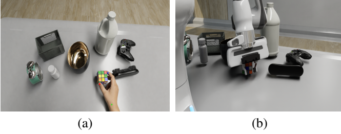
Fig. 5: Rubik's Cube failure case (a) GPT-5.6 Luna generated a grasp from the corner instead of the side. (b) The cube slipped under Franka Panda's finger force, resulting in an unsuccessful grasp.
