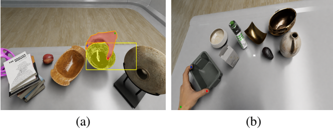
Fig. 6: Failure case examples. (a) Bowl: SAM3 bounding box exceeds object limits causing misplacement of mapped points. (b) Oil Tin: GPT-5.6 Luna incorrectly generated a grasping configuration for a plastic container instead of the oil tin.
