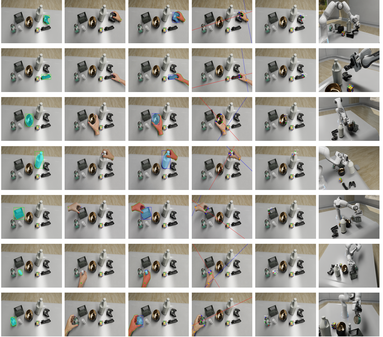
Fig. 3: IMIGRASP: Zero-shot 6-DOF grasp generation using generative AI for imagination guided pose estimation. Each row shows results for one of 7 objects i.e., PS Controller, Shoe Brush, Brass Bowl, Utility Jug, Plastic Container, Packer Bottle, and Alarm Clock. Columns show object mask in actual image, hand grasping image by GPT-5.6 Luna, object and hand masks in genAI image, genAI image with geometric construction lines, object in actual image with final mapped points A, B, T and successful grasp execution attempt by Franka Panda robot respectively.
