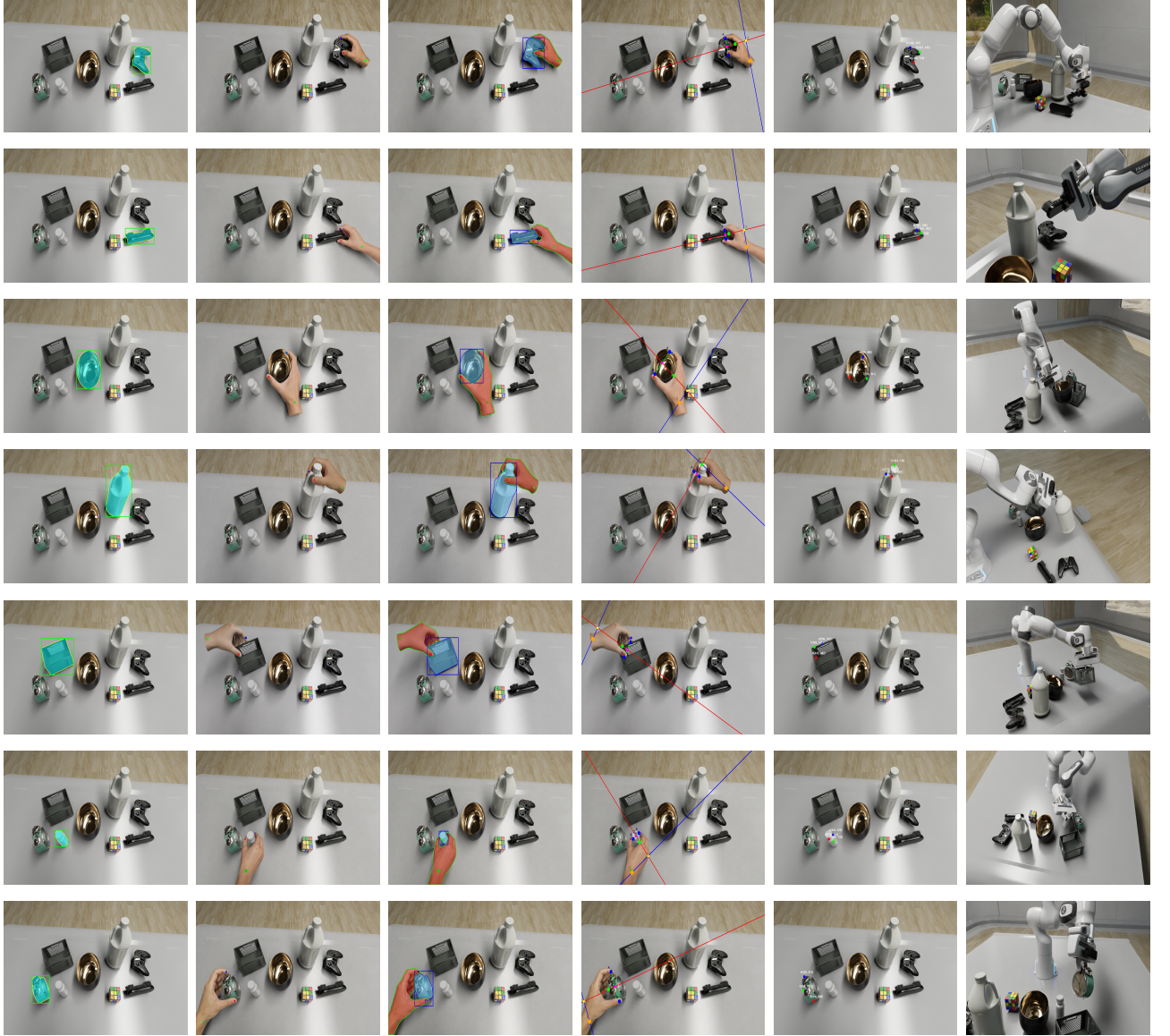
Figure 3: IMIGRASP: Zero-shot 6-DOF grasp generation using generative AI for imagination guided pose estimation. Each row shows results for one of 7 objects i.e., PS Controller, Shoe Brush, Brass Bowl, Utility Jug, Plastic Container, Packer Bottle, and Alarm Clock. Columns show object mask in actual image, hand grasping image by GPT-5.6 Luna, object and hand masks in genAI image, genAI image with geometric construction lines, object in actual image with final mapped points A, B, T and successful grasp execution attempt by Franka Panda robot respectively.
