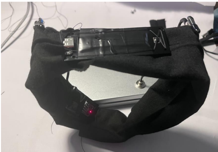
Fig.14 Assembled headband with mounting plates sewn in place
