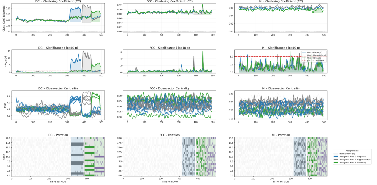
Figure 4. Representative module detection. \text{SCR} = 0.992 . Three sequential coupling modules (DEPRESS, OPPOSEAMP, ELEVATE) occupy the latter half of the record. DCI resolves all three with distinct clustering-coefficient peaks and threshold crossings; PCC and MI miss the events.
