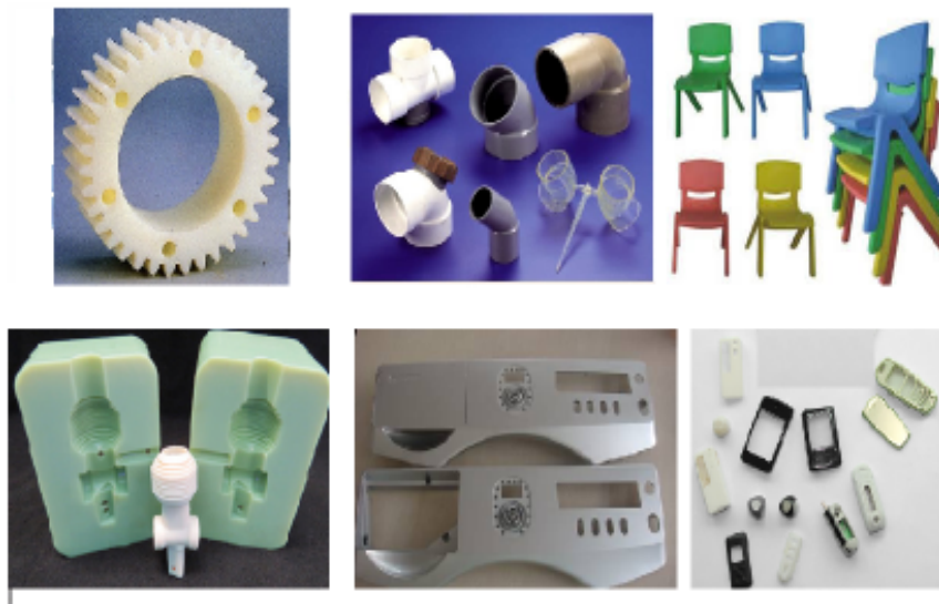
Figure 10.2: Parts produced in injection molding
