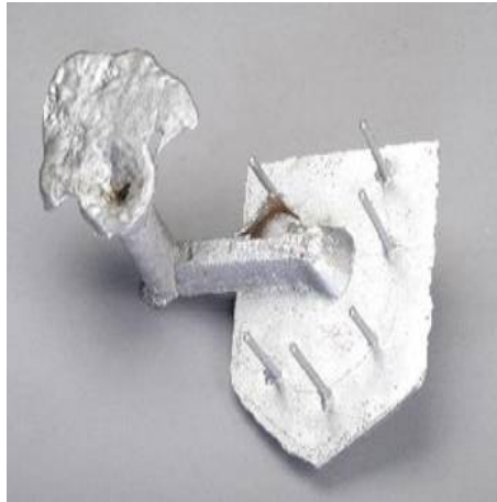
Figure 2.3: A sand casting with risers and the runner system still attached
