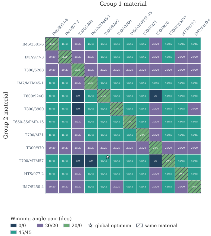
Fig. 17 Fixed-material winning angle-pair matrix for the cutout hardmax landscape. Columns denote the group-1 material and rows denote the group-2 material. Each cell reports the angle pair that gives the lowest objective value for that ordered material assignment. Hatched diagonal cells are same-material assignments, for which same-angle choices are infeasible because identical material-angle groups are excluded from the design library
