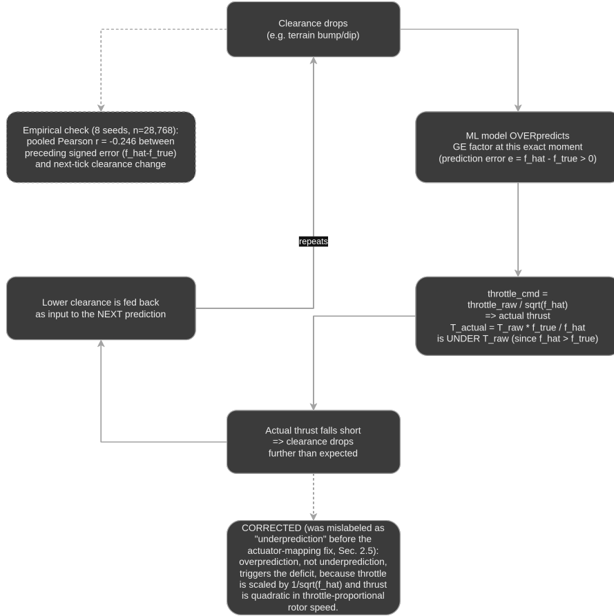
Fig. 19 The causal mechanism verified in Sections 4.5–4.6: transient overprediction of the GE factor causes a measurable, statistically significant degradation in clearance-safety margins (bias intervention), but a pulsed perturbation does not measurably increase subsequent prediction error, and closed-loop pole analysis (below) confirms the system returns to baseline rather than diverging — i.e., the effect is causal but not self-reinforcing.
