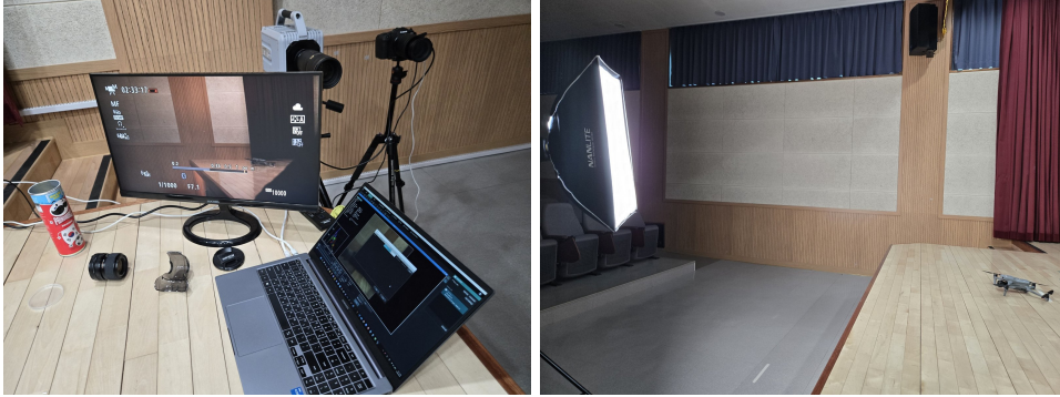
Fig. 1 Pilot observation setup: high-speed camera and reference camera rig (left) and lighting configuration used to permit a high shutter speed at 1000 fps (right).
