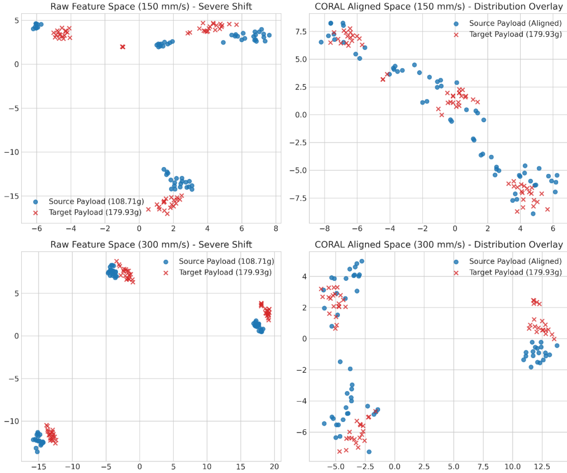
Figure 4: 2D t-SNE projections of raw versus CORAL-aligned feature spaces.
