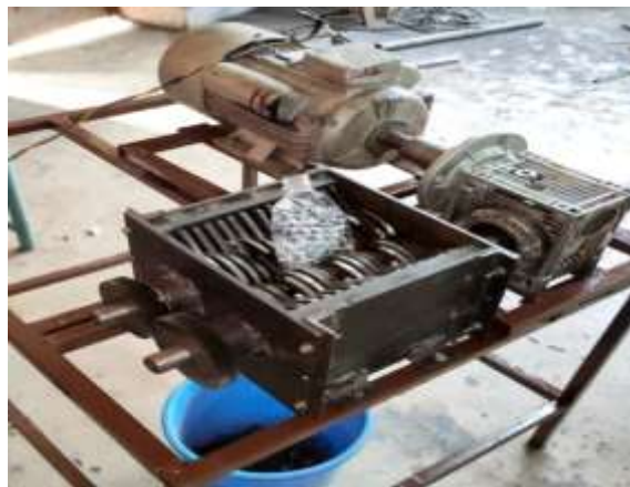
Figure 6.1: Fabricated PET Plastic Shredder
