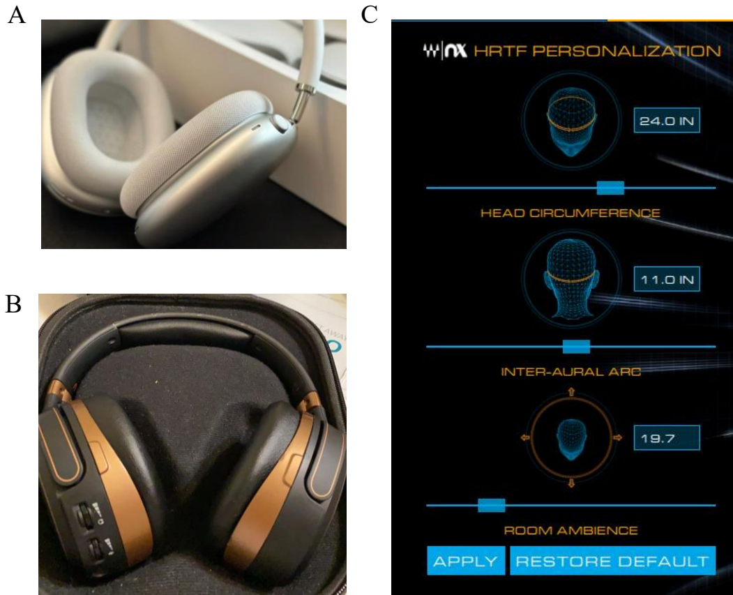
Figure 11. Advanced virtual surrounding headphones using Dolby Atmos or Higher order ambisonics. A: Apple AirPods Max; B: Audeze Mobius and C: HRTF customization setup for Mobius.
