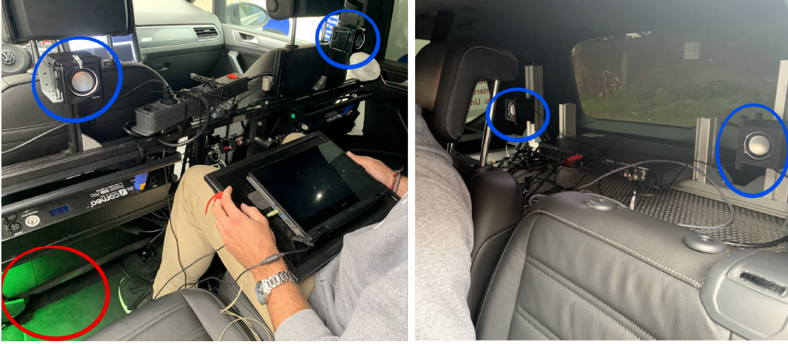
Figure 2: The VISUAL substitution system (red circle; left light bar of the system) illuminated the passenger-side footwell using colored light cues. The AUDIO substitution system (blue circles, 4 of 5 speakers) generated a spatial auditory cue via a dedicated loudspeaker setup (The right light bar and the fifth footwell speaker are not visible in the figure).
