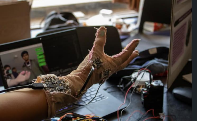
Fig. 2. The instrumented e-textile glove, with embedded piezoresistive sensing and microcontroller hardware at the wrist, shown during a computer-vision hand-tracking session used to validate the landmark-based pose estimation pipeline of Section VI.
