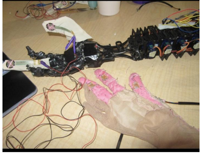
Fig. 1. Benchtop prototype of the tendon-driven robotic hand mechanism. A bank of coupled servo actuators (rear) routes tendons through the fabric-covered finger linkages (front) that reproduce the three principal controllable degrees of freedom described in Section IV.
