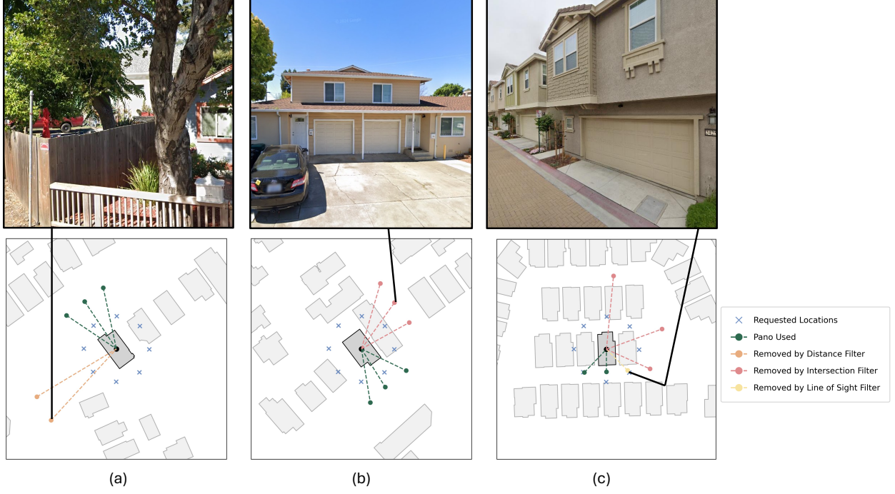
Fig. 2. Image download filters with example images. (a) Distance filter, where the building of interest is too far away; (b) Intersection filter, where the image is clear but does not show the building of interest; (c) Line of sight filter, where the line of sight passes too close to another footprint, creating a misleading view.
