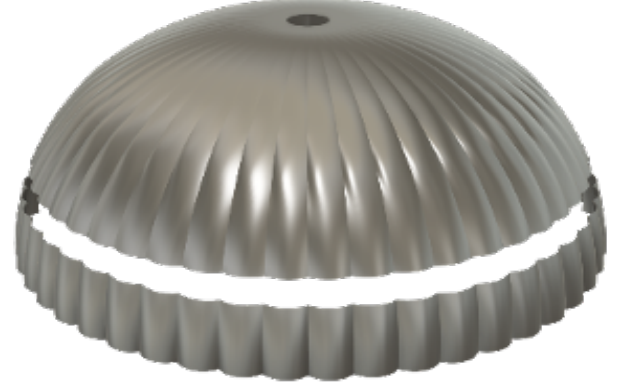
(b) 3D model of DGB parachute used in CFD testing
