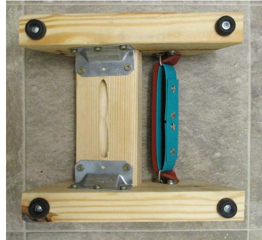
Figure 1. Underside of cradle handle showing joinery
