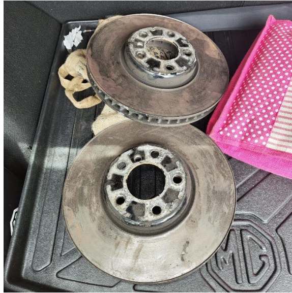
Figure 6 Front rotors of the BMW after testing
