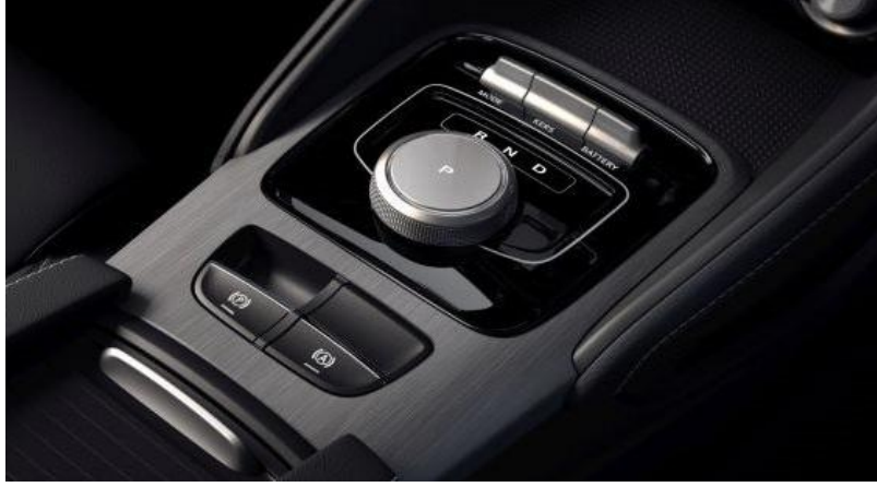
Figure 7 Regenerative braking toggle on the MG ZS EV
