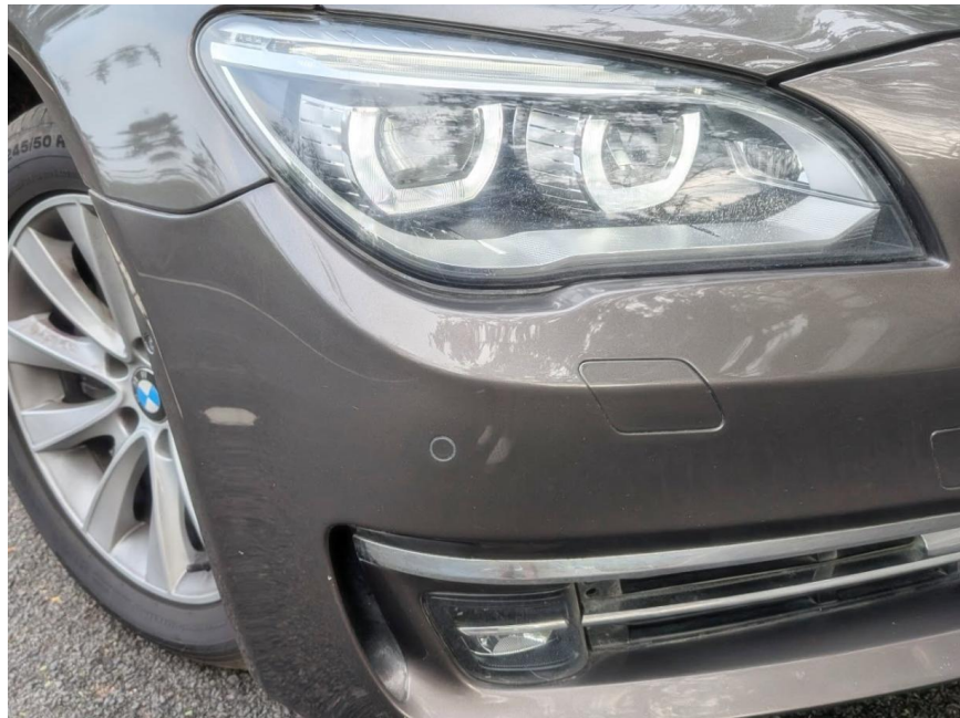
Figure 11 BMW air guides adjacent to fog lights
