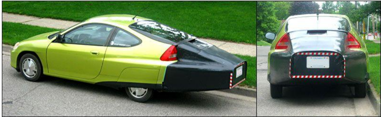
Figure 36 Aerodynamically modified Honda Insight featuring an extended rear for drag reduction.
