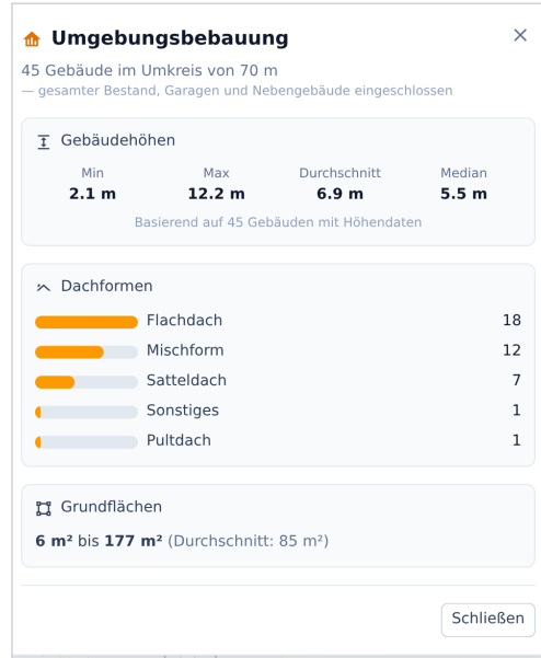
Fig. 2 Statistics of the surrounding buildings derived from open LoD2 data (45 buildings within 70m: heights, roof forms, footprints). Where no development plan exists, such statistics inform the design. Umgebungsbebauung : surrounding buildings; Gebäudehöhen : building heights; Dachformen : roof forms ( Flachdach : flat, Mischform : mixed, Satteldach : gable, Pultdach : mono-pitch); Grundflächen : footprints
