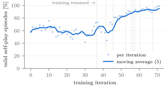
Fig. 11 Share of self-play episodes reaching a valid design per training iteration (dots) and moving average over five iterations (line). Dashed lines mark resumptions of training, partly with code changes, so the improvement reflects both learning and engineering
