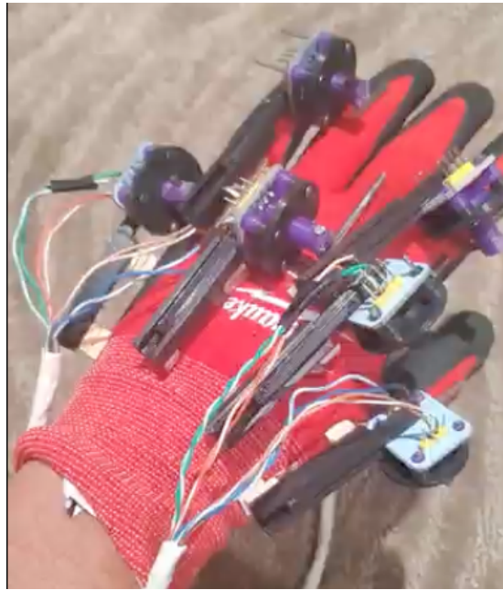
Fig. 2. Dual-joint measurement glove with six magnetic rotary encoders measuring the MCP and PIP joints
