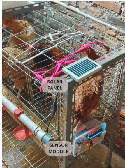
Fig. 3. The device installed on a working chicken coop in a crowded neighbourhood.
