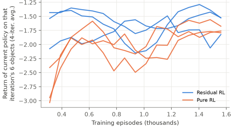
Figure 2: Training curves for three seeds per method. The return of the current policy on each iteration’s six random objects is noisy because the objects change every iteration. Residual RL starts at the model controller’s level because a zero residual is the model controller.
