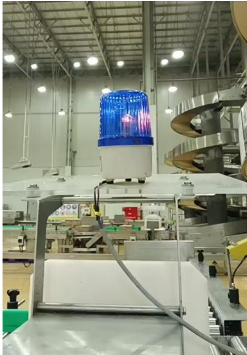
Figure 7. Implementation of the External Visual Alarm on the Coding Box Machine
