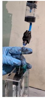
Figure 5. Trial of Cyklop Residual Ink Refill
