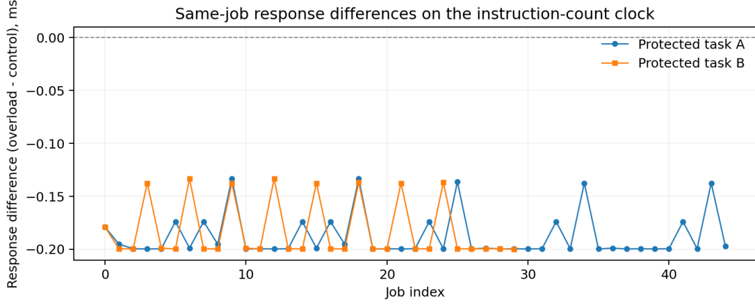
Figure 2: Same-index protected-job response differences between the overload and control boots. Negative numbers are mainly associated with earlier watchdog posts, not a benefit from overload.
