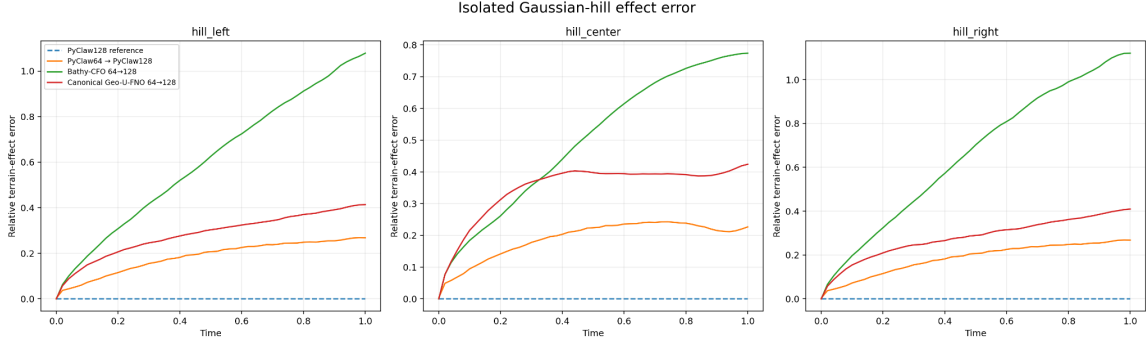
Figure 11: Zero-shot isolated terrain-effect error for left, center, and right Gaussian hills. PyClaw-128 is the zero-error reference. The PyClaw-64 curve is obtained after interpolation to the 128 \times 128 grid.
