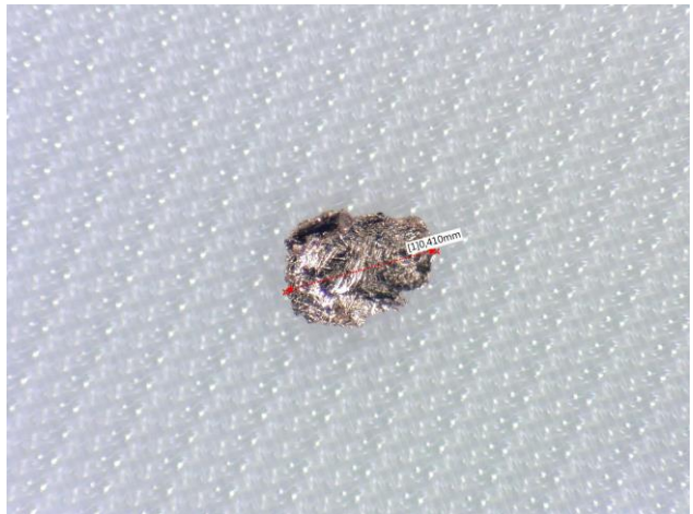
Figures 8-9. Copper particles, from left- bigger, size 0.952 mm; smaller, size 0.410 mm
