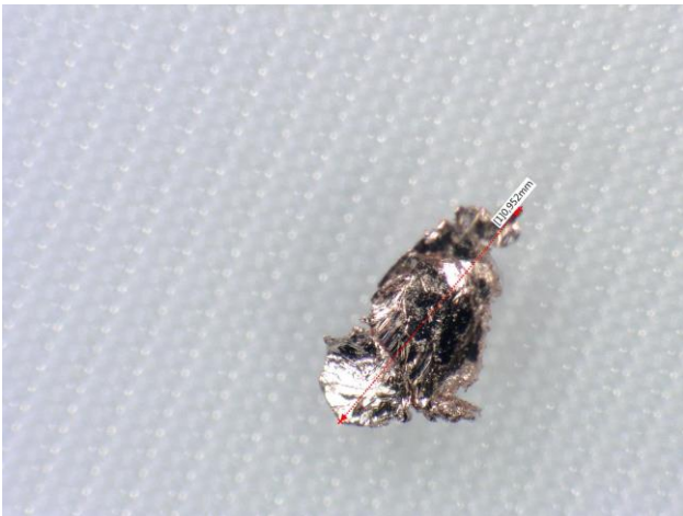
Figures 8-9. Copper particles, from left- bigger, size 0.952 mm; smaller, size 0.410 mm
