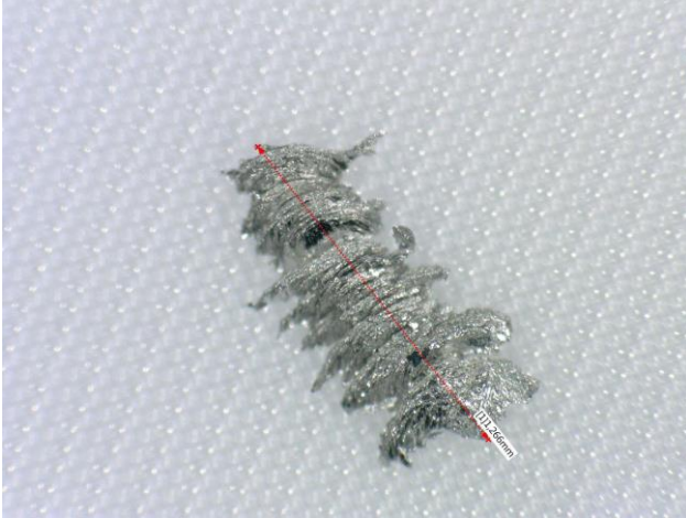
Figures 6-7. Tin particles, from left- bigger, size 1.266 mm; smaller, size 0.729 mm
