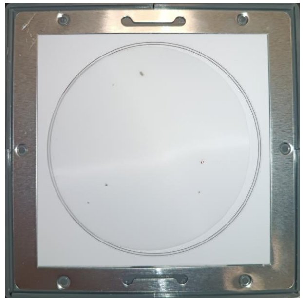
Figure 2. Positioning of particles of Tin (topmost), Copper (bottom right) and Aluminium (bottom left)
