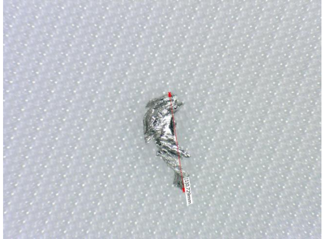
Figures 6-7. Tin particles, from left- bigger, size 1.266 mm; smaller, size 0.729 mm
