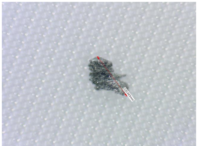
Figures 10-11. Aluminium particles, from left- bigger, size 0.723 mm; smaller, size 0.443 mm
