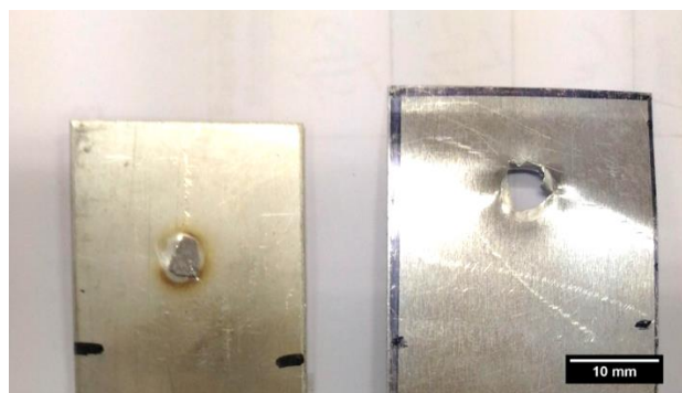
Figure 4: Image of tensile test sample after fracture (weld current = 4 kA, weld time = 8 s).
