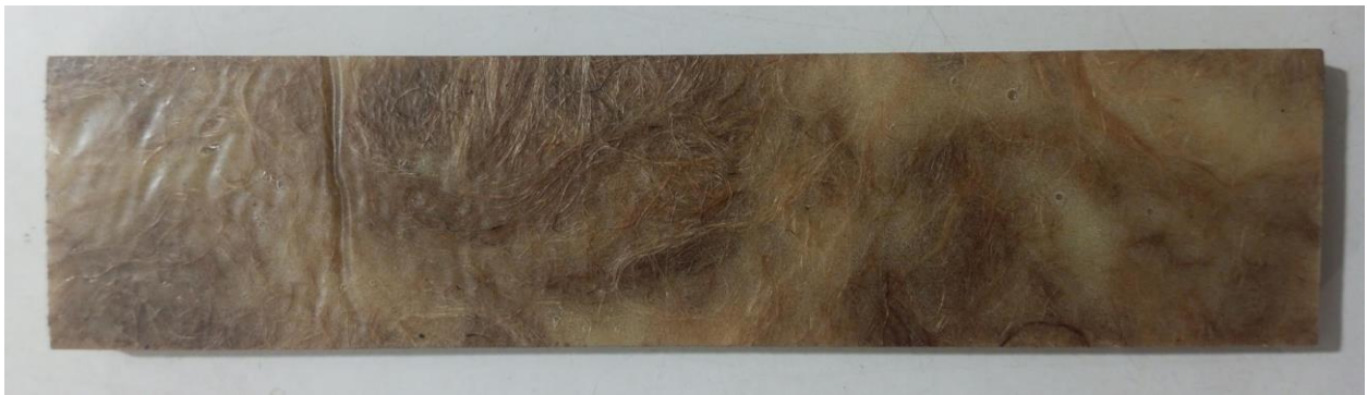
Figure 4.1: Sample Composite Board Mixture of Coconut Fibers and Jute Fibers
