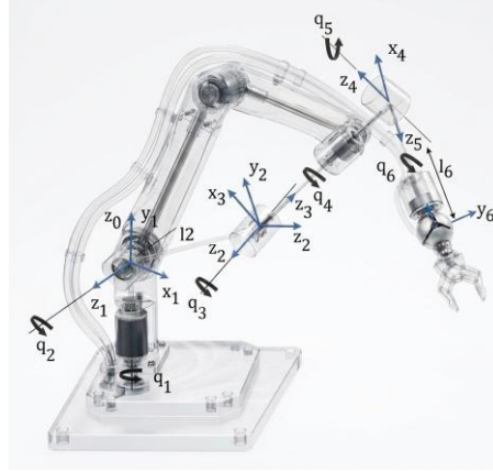
Figure 1. Schematic of the 3-DOF wrist-center positioning model derived from the 6-DOF anthropomorphic arm with spherical wrist. Only joints q_1, q_2, q_3 affect the wrist-center position; joints q_4, q_5, q_6 control orientation and are not addressed in this study.
