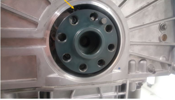
Figure 4: Flywheel side of the engine without installed crankshaft seal
